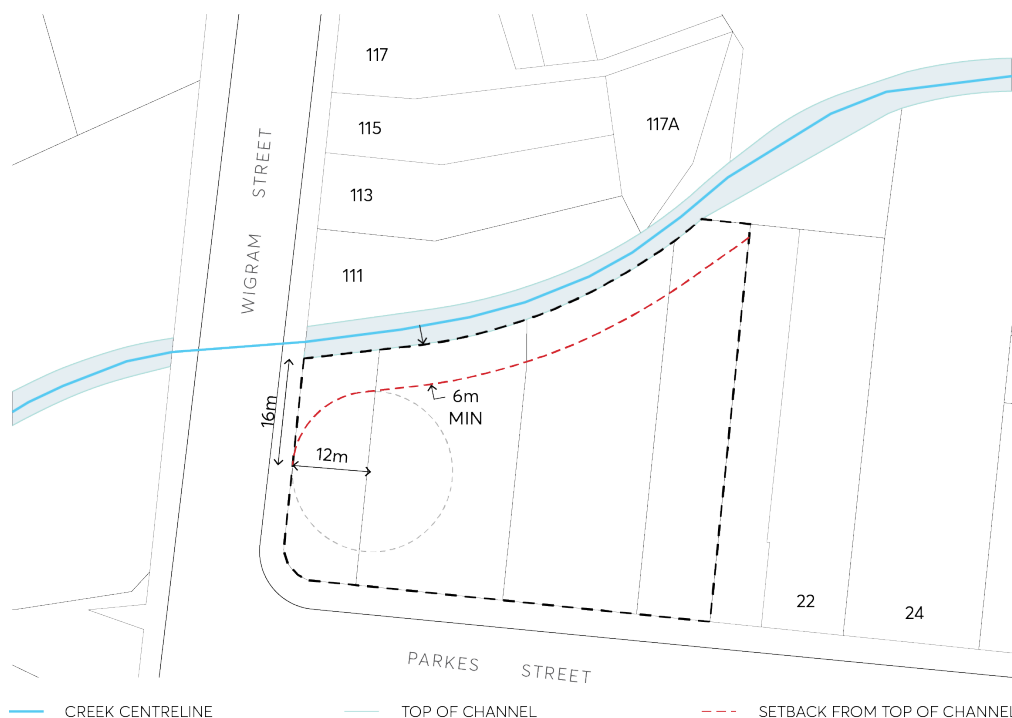
Figure 9.10.8.2 – Required floodway setbacks
