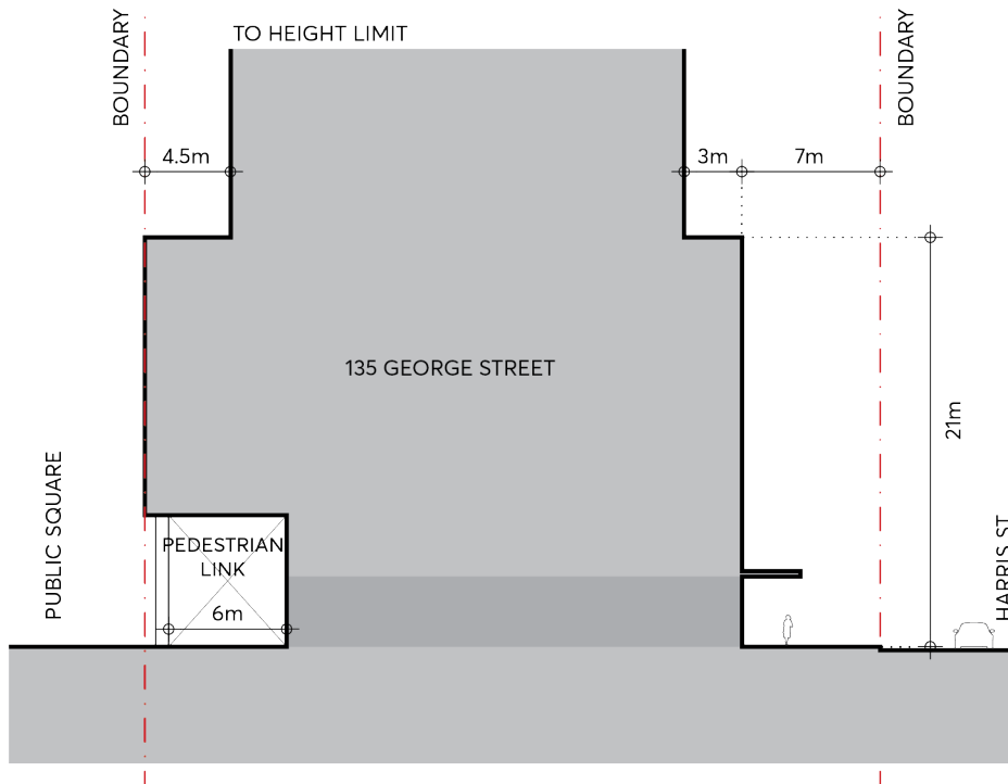
Figure 9.10.10.7 – Section showing double height colonnade and setbacks to tower at the corner of Harris and George Streets
