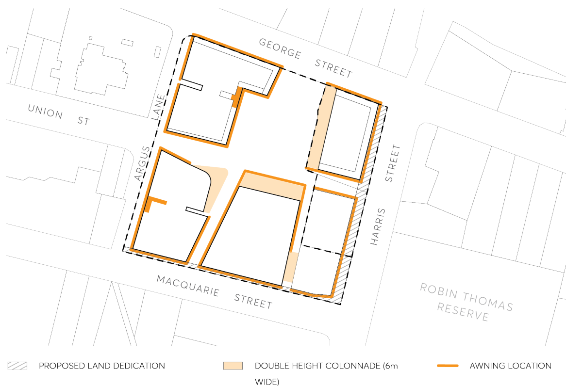
Figure 9.10.10.4 – Awning location for former Cumberland Media and Albion Hotel sites
