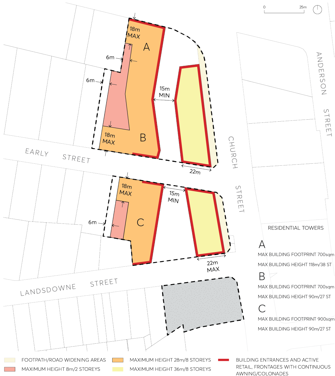
Figure 9.10.2.3 – Building Form Control Plan
