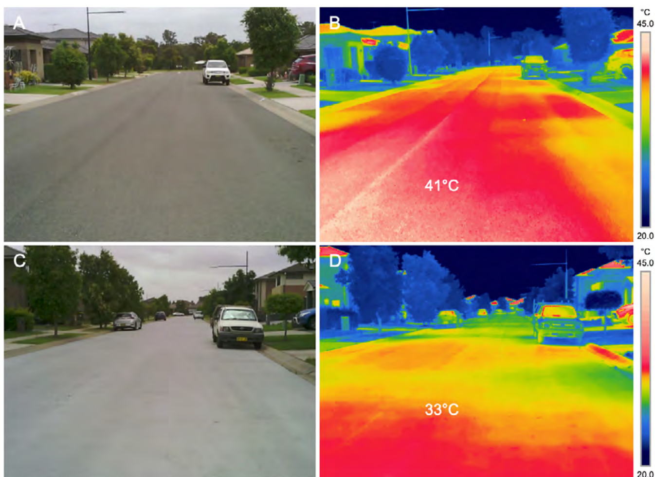
FIGURE 14: Surface temperature during overcast conditions. The images were taken on 2 December 2020 at Mackey Circuit (A, B) and Kobe Street (C, D) in Ropes Crossing, Blacktown LGA. Panels A and C show normal views, panels B and D show infrared views where different colours represent different surface temperatures (see scale on right side).
