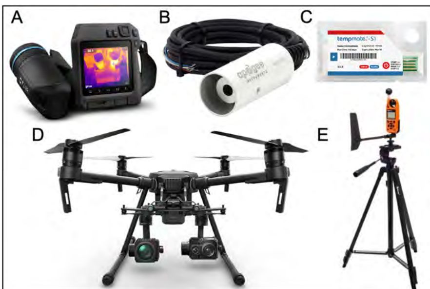
FIGURE 7: Instruments used to monitor a range of temperatures during the Cool Roads Trial. A: FLIR T540, hand-held radiometric infrared camera for on-ground spot measurements of surface temperature. B: Apogee T400 radiometer for continuous measurement of surface temperature. C: Tempmate S1 V2 temperature sensor for continuous measurement of ambient air temperature. D: DJI M210 aircraft and FLIR Zenmuse-XT2 for aerial spot measurements of surface temperature. E: tripod-mounted Kestrel 5400 Heat Stress Tracker with black globe thermometer as proxy for human thermal comfort.
