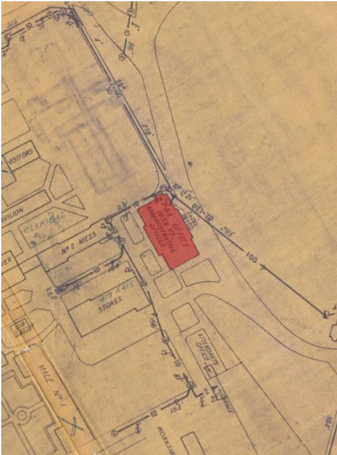
A-13 An excerpt of a 1959 electrical services site plan for the Parramatta Mental Hospital. The former Visitor's and Administration Block is noted here as 'Administrative Offices'. Note also that the Criminal Asylum Ward and its walled enclosure is shown demolished, suggesting that the plan was modified in the mid-1960s. Source: tbc, with TKD Architects overlay, 2016.
