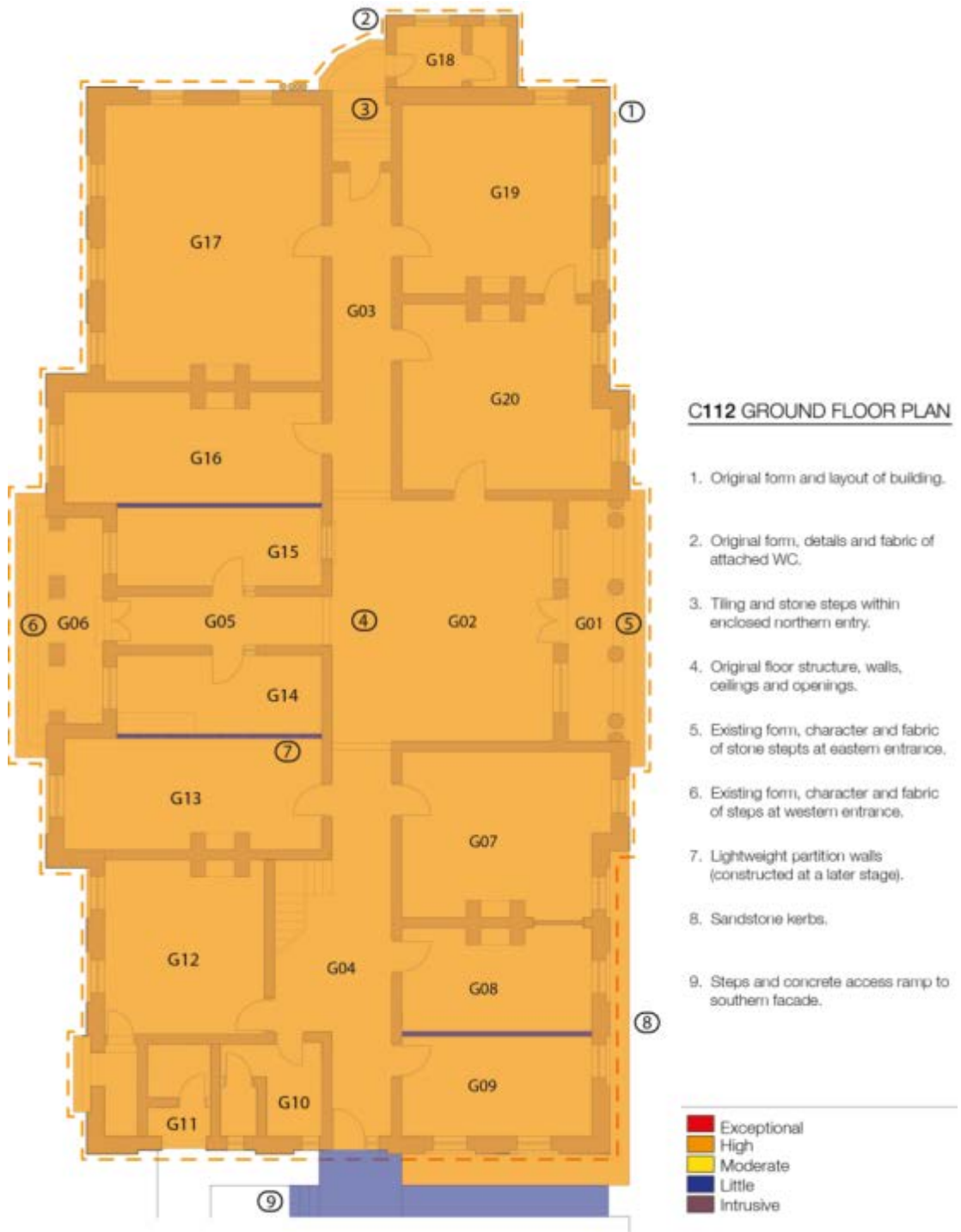
A-23 The ground floor plan of the Mental Health Sciences building illustrating the significance of various spaces, components. Source: TKD Architects, 2016.
