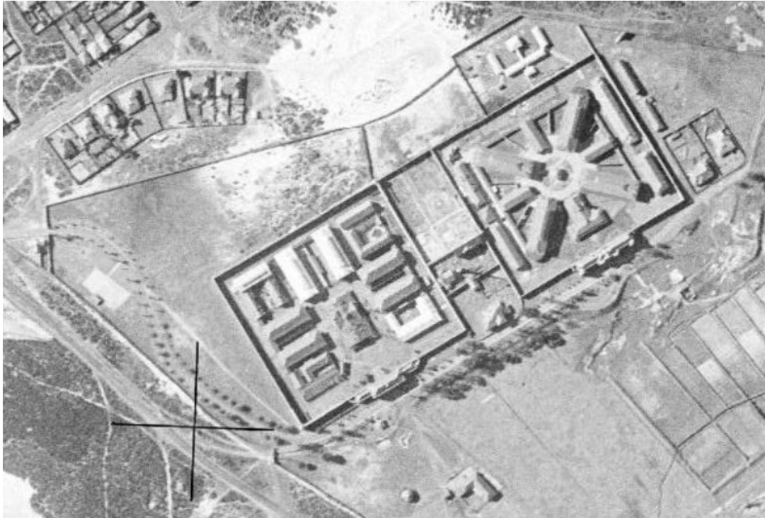
82 Aerial photograph of Long Bay Gaol, 1943. The radial layout of the Female Reformatory contrasts with the regular grid-like layout of the Male Penitentiary Source: Spatial Information Exchange.
