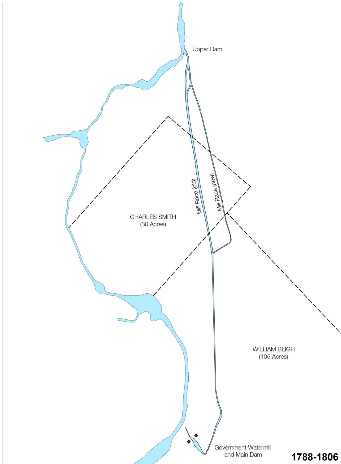
B-1 The PNHS in 1806 illustrating the 1792 land grant to Charles Smith, the land grant to Governor William Bligh and the establishment of the Government watermill and associated dams and mill races. The locations for the mill, mill races and upper dam are approximate only. The upper dam and north end of the mill races are located within the boundaries of Parramatta Gaol site established in the 1890s—in particular Precinct 2—Gaol Farm/Linen Service and Precinct 5—Riverfront/Riparian Corridor. Source: TKD Architects, 2016.
